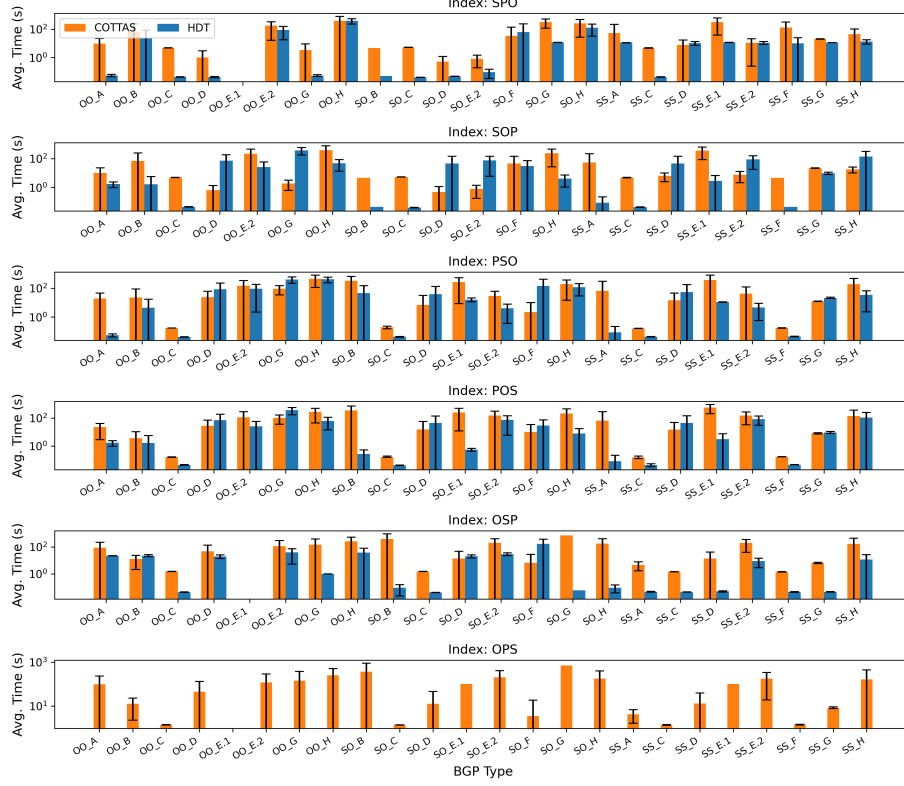
Fig. 6: Average execution time for the different type of big joins and indexes over the DBpedia dataset in the COTTAS and HDT formats. Time is reported in seconds using log scale. Bars are missing for indexes that failed in their creation.
